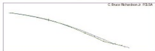
Figure 3: Lens profile showing how the peripheral curves of the lens differ from the initial contact lens design and the final contact lens design. (Copyright of Eastern Contact Lens)
